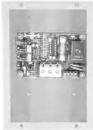
These voltage controlled switches are activated when the battery bank voltage reaches a user adjusted set point. The "Activate High" model is commonly used to turn on a battery vent fan. The "Activate Low" model can be used as a load controller. Both versions work
